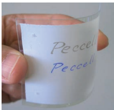
Figure 7. Mesoporous TiO 2 -coated ITO-PEN film as working electrode for dye-sensitization. The TiO 2 layer shows high hardness against writing by pencil (upper) and ball-point pen (lower). Electrode thickness, 210 μm including 10 μm-thick TiO 2 layer.
